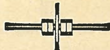
EC 9. Loose Wheel. Consisting of:— 1 × S 25 or S 55 4 × N 1 1 × P 29 or W 10 or W 16
