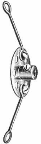
Fig. 4.—Spokes bent for standard wheel.
