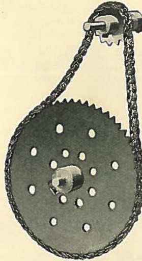
S.M. 7—Chain Gear \frac{3}{4} " and 3 " diam. Sprocket Wheels. Ratio, 4 : 1. 1" and 2" diam. Sprocket Wheels. Ratio, 2 : 1. \frac{3}{4} " and 1\frac{1}{2} " diam. Sprocket Wheels. Ratio, 2 : 1. etc., etc. Ratios of 1 : 1 may be obtained by gearing any two Sprocket Wheels of like diameter
