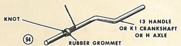
94 METHOD OF TYING A STRING ON HANDLE, CRANKSHAFT OR AXLE
