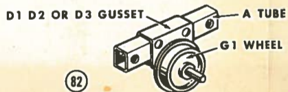
82 AXLE FIXED THROUGH THE HOLES OF A GUSSET
