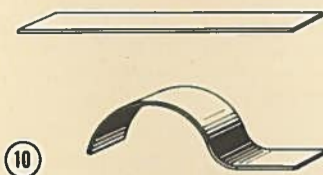
10 HOW A PLATE MAY BE BENT TO FORM A FENDER
