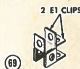
69 ATTACHING 2 E1 CLIPS AT RIGHT ANGLES
